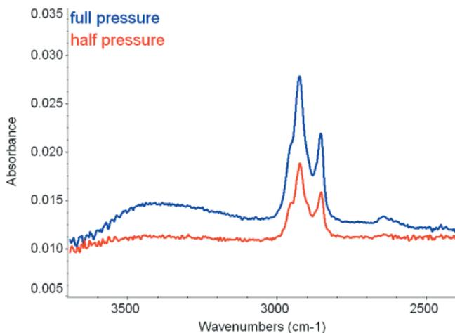
**Figure 3. Effects of varying applied pressure (full and half) on spectral quality.**
