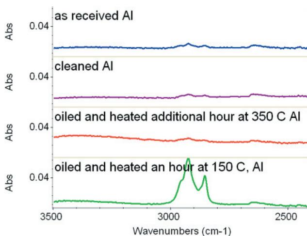
**Figure 4. Spectral comparison of aluminum sample treatments, shown at identical y-scaling.**
