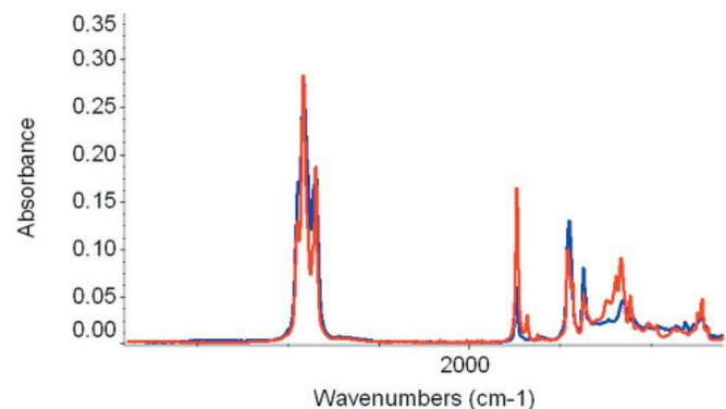
Figure 2. Spectra of two aluminum cutting fluid brands.
