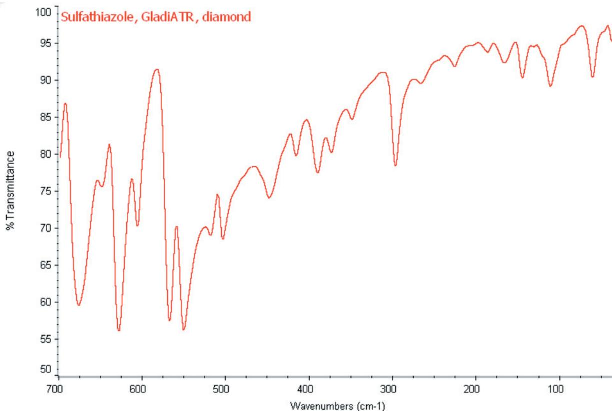
**Figure 2.** Sulfathiazole powder measured by ATR/FTIR using the GladiATR accessory with diamond crystal plate.
