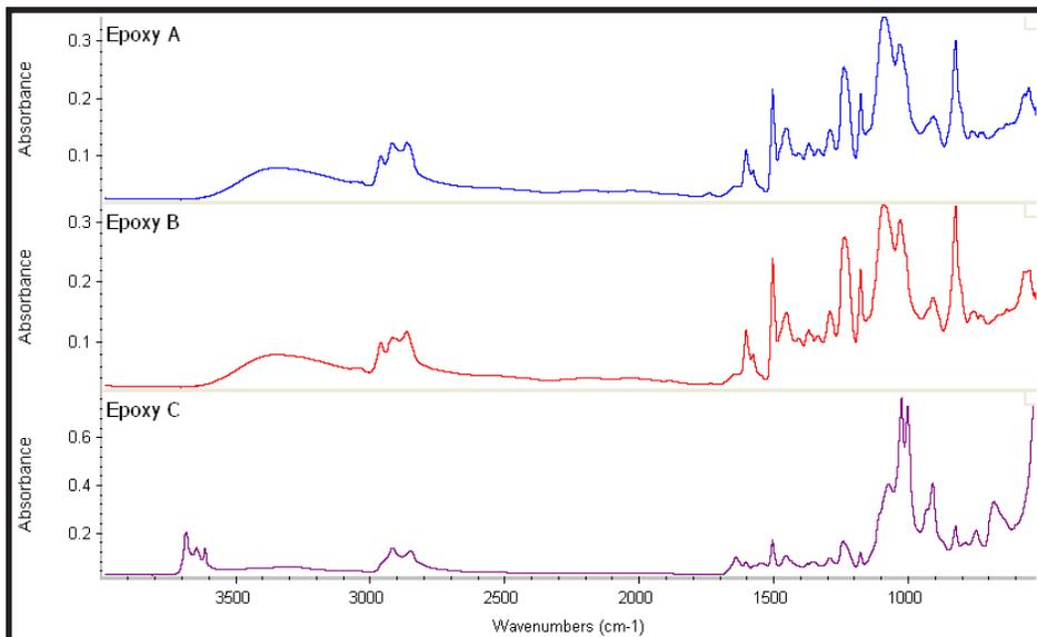
**Figure 2:** ATR / FTIR Spectra for Cured Epoxy Samples from 3 Different Manufacturers.
