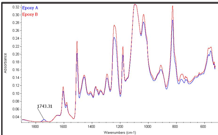
**Figure 3:** Expanded Fingerprint Region for Epoxy Samples A and B.
