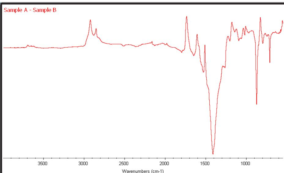
**Figure 5.** Subtraction Result for Cured Epoxy Samples A Minus B.
