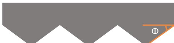
A 2<sup>nd</sup> generation SEIRAS-optimized wafer was designed with a greater groove face angle (55° compared to 35°) compared to a previously reported 1<sup>st</sup> generation Single Reflection ATR wafer. For both wafer generations, Table 1 lists the face angles and range of AOI at the electrode-solution interface, AOI<sub>ESI</sub>, which results from incoming light at AOI<sub>inc</sub>.
