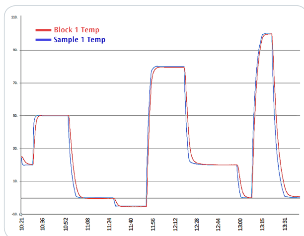
Accessory performance showing block temperature (red) and sample probe temperature (blue).
