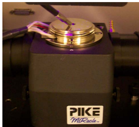
Fig.1 PIKE Miracle™ with heated diamond ATR crystal. UV source with 254nm and 365nm was placed above the sample in close proximity.
