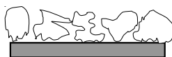
Figure 3 An example of the difficulty of getting crystallites of powdered sample to make good contact with an ATR crystal surface.
