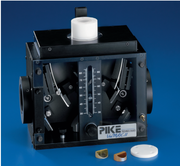
Spectroelectrochemical cell with removable and interchangeable crystals mounted on the VeeMAX
