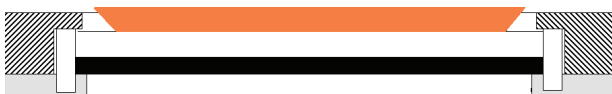
Flat plate HATR crystal plate – ideal for solids, polymer films and coatings
