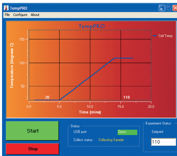
PIKE TempPRO Software for Kinetic Experiments with our Resistively Heated Crystal Plates
